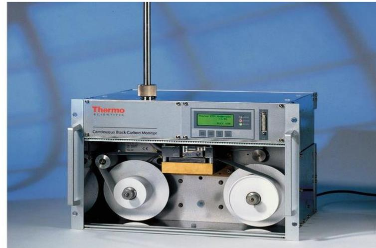
Figure: Model 5012 MAAP Detection Chamber and Instrument itself
